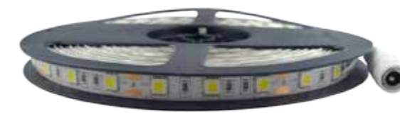
H-TLED-60-IP65-5050 Tira flexible de LED 5050 SMD 12V IP65: uso exterior, 60 LED/M Requiere driver de 12V
